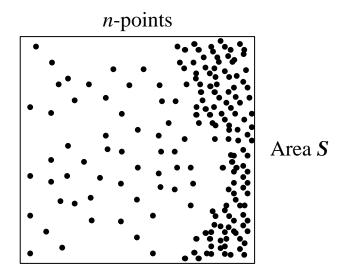
$$-\Pr\{N(S) = n\} = \frac{\left(\int \int_{S} \lambda(x,y) dx dy\right)^{n}}{n!} e^{-\int \int_{S} \lambda(x,y) dx dy}$$
