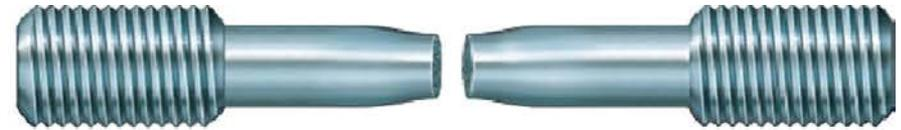
Failure of a ductile material
