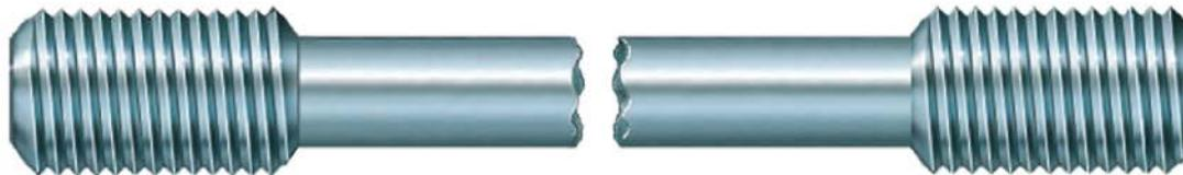
Tension failure of a brittle material
